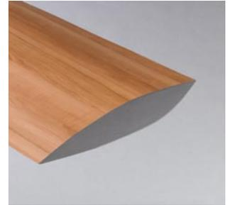
EGGER Laminate MED is a decorative laminate based on curable resins. The laminate is constructed by fusing multiple layers and consists of melamine resin impregnated decor paper and several phenolic resin impregnated core layers. EGGER Laminate MED is suitable for all uses / areas of application as outlined below and in addition meets the requirements of the **Marine Equipment Directive** with regard to:
